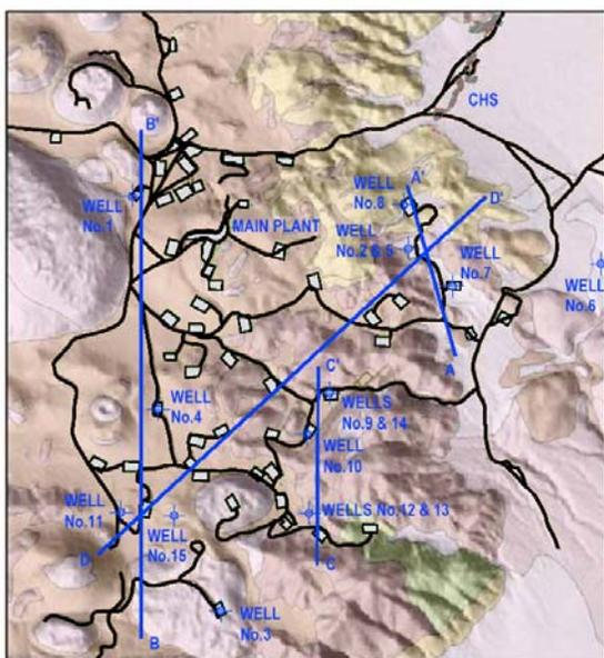
Figure 1. Map of the Coso Geothermal Field showing the cross-section and well locations (After Moore, 2005).
