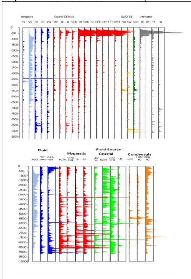
Figure 2: Well logs for Well 2. Note the large organic peaks near the surface indicating shallow meteoric fluids and the high  $N_2/Ar$  and  $CO_2/CH_4$  ratios at depth indicating reservoir fluids.
