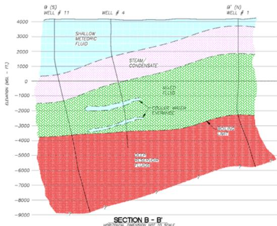
Figure 4: Cross-section based on FIS of the western edge of the Coso field. Well 1 is to the north end of the field.
