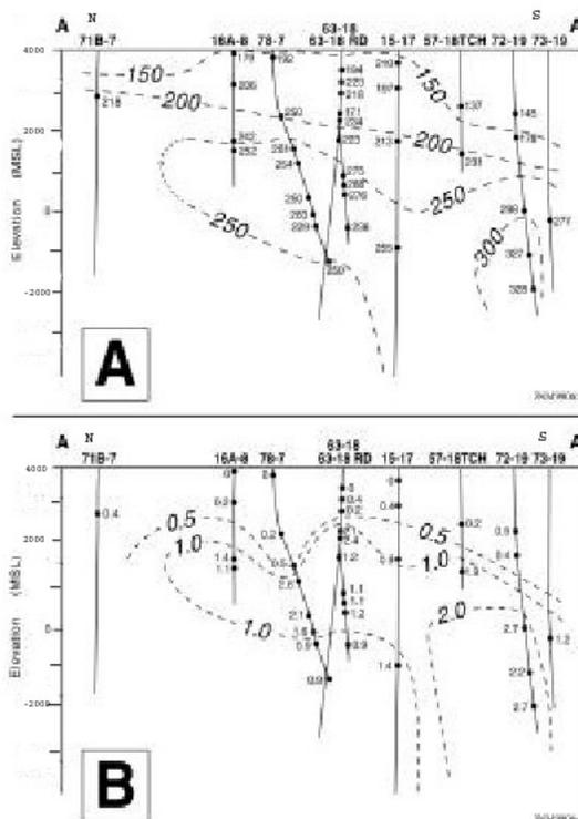
Figure 5: North-south cross-sections of the reservoir prepared based on fluid inclusion studies in 1999/2000 in Adams et al, 2000. A) Maximum fluid-inclusion homogenization temperatures and B) maximum salinities of inclusion in weight percent NaCl equivalent. A on the cross-section is to the north and A' is to the south.
