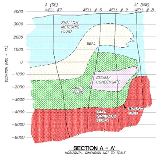
Figure 3: Cross-section based on FIS of the East Flank area.
