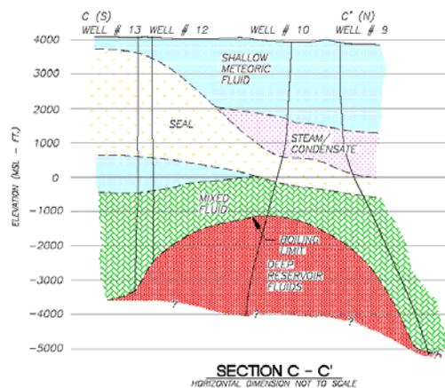
Figure 6: Cross-section based on FIS of the middle southern portion of the Coso field.
