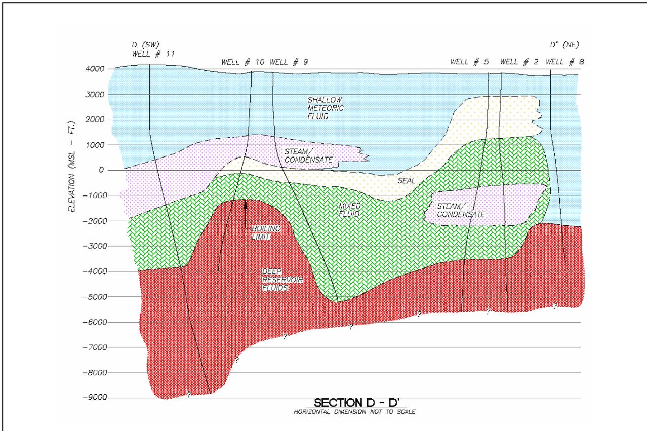
Figure 7: Cross-section based on FIS diagonally across the Coso field from the southwest to the northeast.
